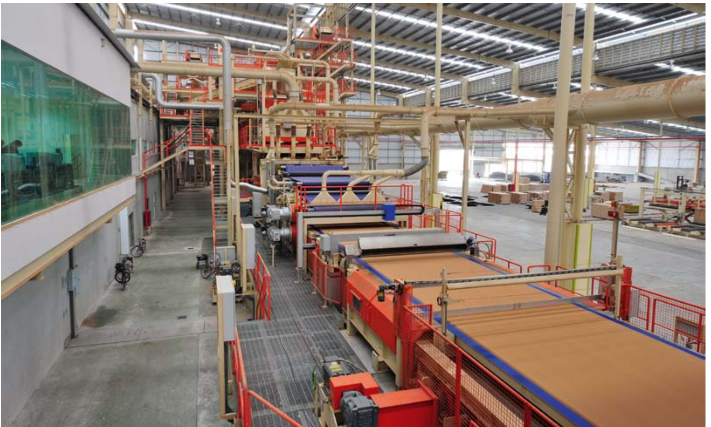
Forming line of a particleboard plant
